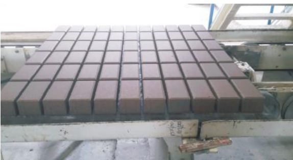
Blocks produced in an automated unit using LC 3 in Ghaziabad
